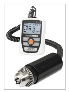
Series TT03 digital torque gauges are designed for clockwise and counter-clockwise torque testing applications in virtually every industry, with capacities from 10 ozFin to 100 lbFin (7 to 1,150 Ncm). A dedicated remote torque sensor with Jacobs chuck can be used to grip a sample, bit, or fixture. The gauges' rugged aluminum housing allows for hand-held use or test stand mounting for more sophisticated testing requirements.
