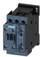
power contactor, AC-3 12 A, 5.5 kW / 400 V 1 NO + 1 NC, 42 V AC, 50 Hz 3-pole, Size S0 screw terminal
