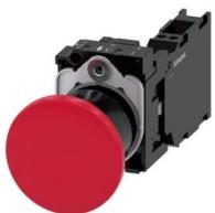
Mushroom pushbutton, 22 mm, round, plastic, red, 40mm, latching, pull-tounlatch mechanism, with holder, 1 NO+1 NC, spring-type terminal, with laser labeling, symbol number according to, ISO 7000 or IEC 60417
