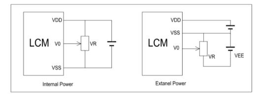
VDD-V0: LCD Driving Voltage VR: 10k-20k
