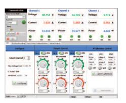
PC software is provided for front panel emulation, generating and executing test sequences or logging measurement data without the need to write source code.
