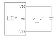
VDD~V0: LCD Driving voltage
