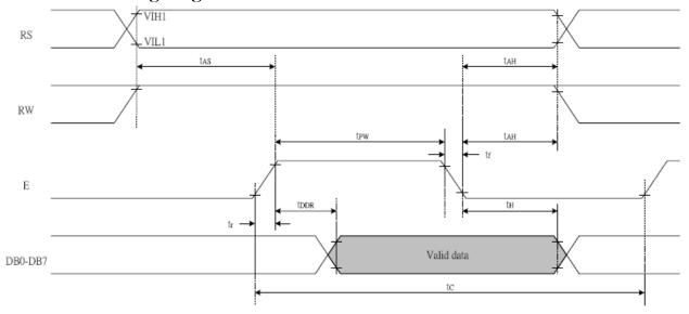
Write cycle (Ta=25°C, VDD=5.0V)
