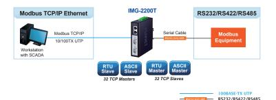
The advantage of having the IMG-2X00T Series is to assist users to build an industrial environment between the Modbus TCP/IP Protocol and the Modbus RTU/ ASCII Protocol easily, thus offering an application solution to the industrial control equipment without Ethernet ports and the industrial control equipment can only
