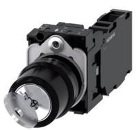
RONIS key-operated switch, 22 mm, round, plastic, lock number SB30, with 2 keys, 2 switch positions O-I, latching, 10:30h/13:30h, key removal O+I, with holder, 1 NO+1 NC, screw terminal, possible special locks: SB31, 421, 455
