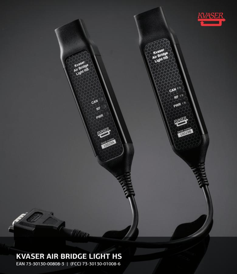
Kvaser Air Bridge Light HS is a configuration-free wireless CAN bridge that achieves predictable latency, without sacrificing stability or range. Comprising a preconfigured pair of plug-and-play units to exchange raw CAN data, the Kvaser Air Bridge Light HS is designed for environments or situations that make wired connection unsuitable or challenging e.g., between two moving parts that are connected by CAN.
