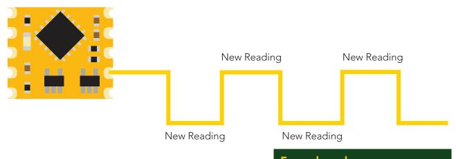
The pin will automatically invert its state each time a new reading is available. This setting has been specifically designed for a master device that can use an interrupt on change function.
