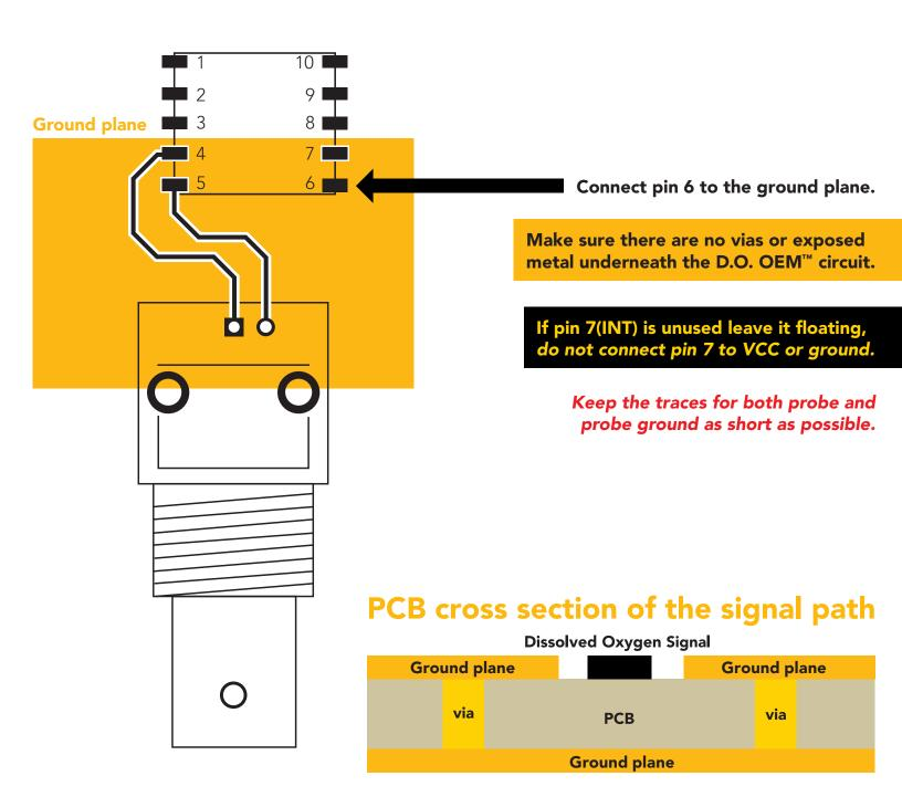
This cross section is an example of how the ground plane protects the Dissolved Oxygen signal. The ground plane should surround the Dissolved Oxygen signal, on the top layer as well as the bottom layer.
