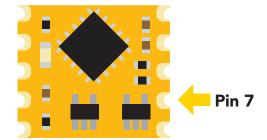
The Interrupt control register adjusts the function of pin 7 (the interrupt output pin).
