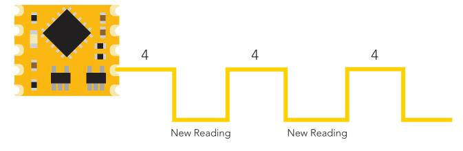
The pin will not auto set. 4 must be written to the interrupt control register after each transition from high to low.
