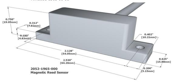
All measurements are in Inches [millimeters]
