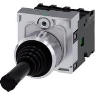
Coordinate switch, 22 mm, round, metal shiny, black, 4 switch positions, momentary contact type, without mechanical interlocking, in O position, with holder, 1 NO, 1 NO, 1 NO, 1 NO, screw terminal, Z=20-unit packaging
