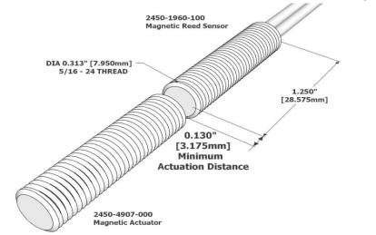
All measurements are in Inches [millimeters]
