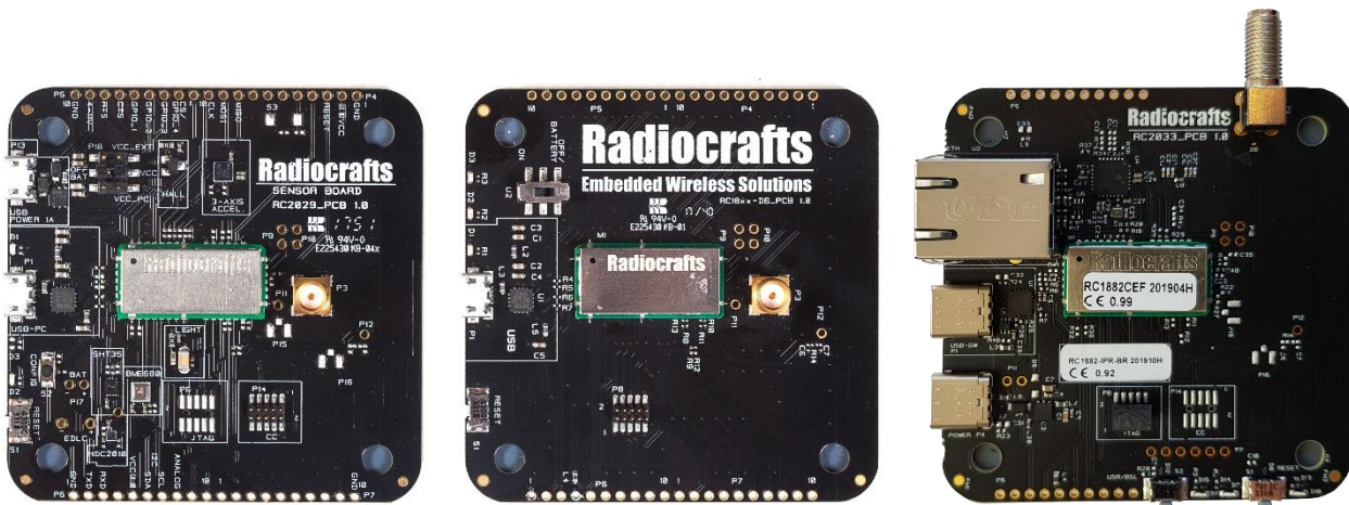
Figure 2. Sensor board(left) and development board(middle) and border router board(right)
