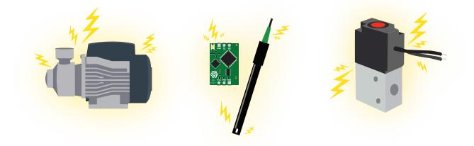
When reading pH and Conductivity or Dissolved Oxygen together, it is **strongly recommended** that the EZO<sup>™</sup> pH circuit is electrically isolated from the EZO<sup>™</sup> Conductivity or Dissolved Oxygen circuit.
