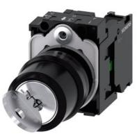
RONIS key-operated switch, 22 mm, round, plastic, lock number SB30, with 2 keys, 2 switch positions O-I, latching, 10:30h/13:30h, key removal O+I, with holder, 1 NO, screw terminal, possible special locks: SB31, 421, 455, with laser labeling, upper case
