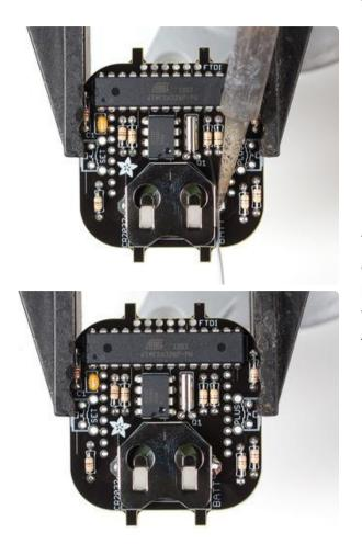
The battery holder will slip out if you flip over the board, so before flipping the board, solder one leg side from the top. The holder is a great heatsink so it may take a little longer than usual to solder in
