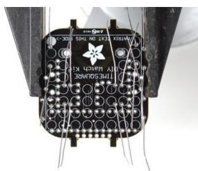
You did great with the first two parts, now we will solder in the remaining resistors R1-R8. These resistors are the LED 'choke' resistors - they keep the LED matrix's light even and avoids having too much current draw that would kill the battery off!
