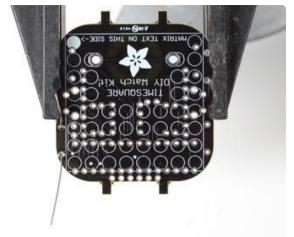
With your soldering iron heated up and ready, solder in both leads of the resistor. To do this, heat up the round ring pad and the wire lead at the same time for 2 or 3 seconds, then dip the end of the solder into the heated joint to melt it in.
