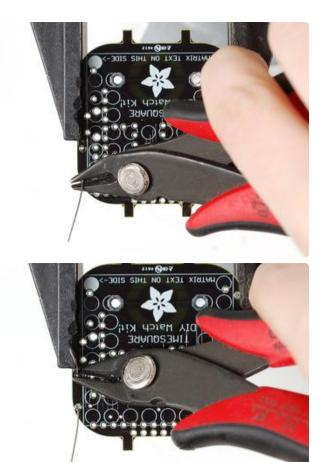
Once the soldering is complete, we can clean up by clipping the leads of the resistor. This keeps them from shorting to something else. Use diagonal or flush cutters to clip the wires right above where the solder joint ends.
