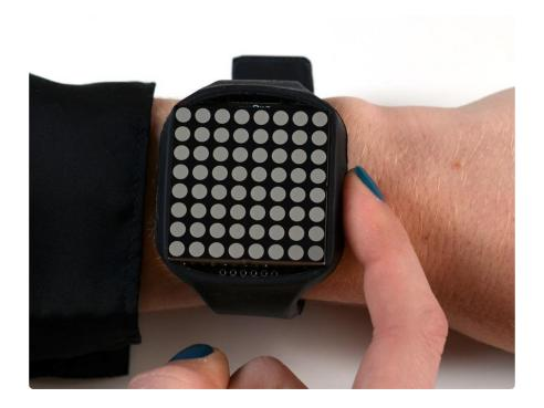
There are two digits each for the year, month, day, hour and minute, and the watch will briefly display the symbols Y, M, D, etc. when moving from one pair of digits to the next. The high and low digits are set individually...this is different from most digital clocks, we find it faster and less troublesome. The range for each digit varies, and the watch will keep the values in check.
