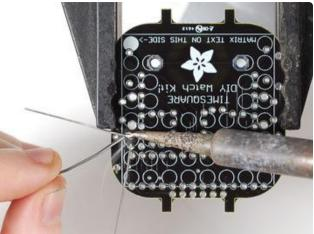
Solder in the capacitor's two legs just like you did with the resistor
