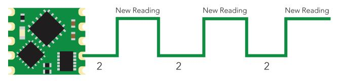
The pin will not auto reset. 2 must be written to the interrupt control register after each transition from low to high.
