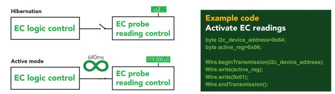
Once the device has been woken up it will continuously take readings every 640ms. Waking the device is the only way to take a reading. Hibernating the device is the only way to stop taking readings.
