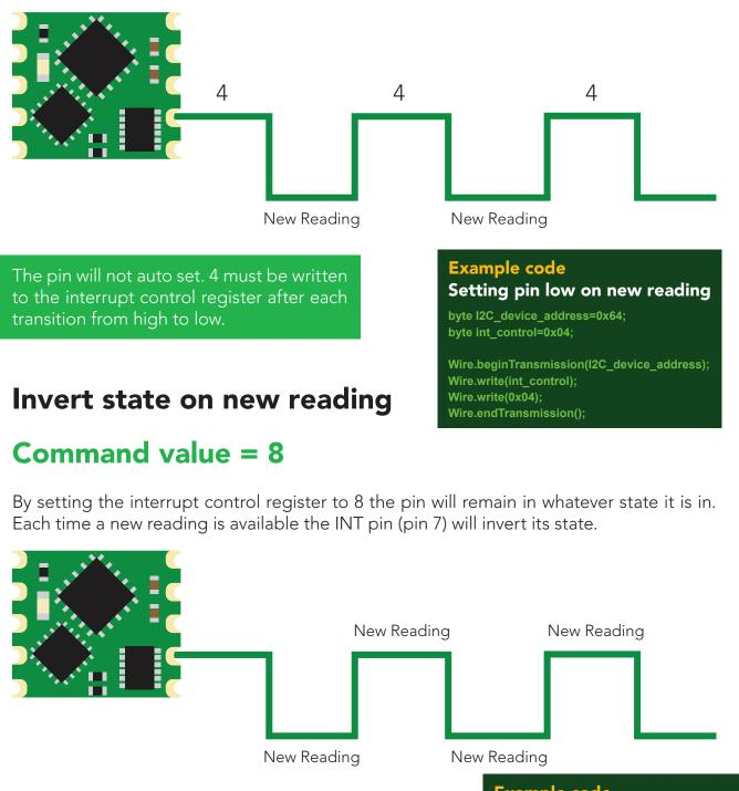
The pin will automatically invert its state each time a new reading is available. This setting has been specifically designed for a master device that can use an interrupt on change function. Example code
