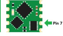
The Interrupt control register adjusts the function of pin 7 (the interrupt output pin).
