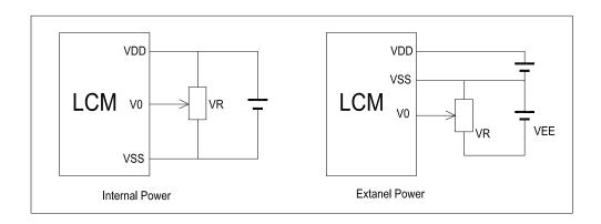
$V_{\text{DD}\text{-}}V_0\text{: LCD}$  Driving voltage
