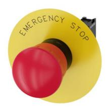
EMERGENCY STOP mushroom pushbutton, 22 mm, round, plastic, red, 40 mm, positive latching, acc. to EN ISO 13850, rotate-to-unlatch, with yellow backing plate, inscription: EMERGENCY STOP, with holder, 1 NC, screw terminal
