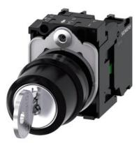
RONIS key-operated switch, 22 mm, round, plastic, lock number SB30, with 2 keys, 3 switch positions I-O-II, latching, 10:30h/12h/13:30h, Key removal I+O+II, with holder, 1 NO, 1 NO, screw terminal, possible special locks: SB31, 421, 455, with laser labeling, upper case and lower case, always upper case at the beginning of the word
