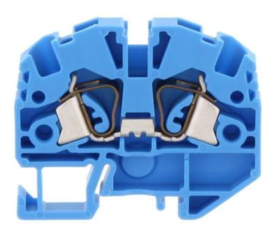
Feed-through terminal, Tension-spring connection, Mounting type: Mounting rail TS 15/5.5, Rated cross-section: 2.5 mm², Width: 5.1 mm, Colour: Blue
