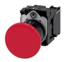
Mushroom pushbutton, 22 mm, round, plastic, red, 40mm, latching, pull-to-unlatch mechanism, with holder, 1 NC, screw terminal, Z=20-unit packaging
