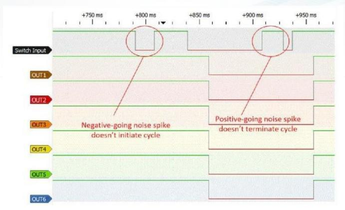
This logic analyzer capture of a LS10 Series IC cycle showing a noisy switch input commonly applied to all six device channels. Note the initial 19 ms High-going glitch at approximately +780 ms does *not* start a cycle, and the folHighing 18 ms high-going first glitch at about approximately +915 ms does *not* terminate the cycle. LS10 Series devices are designed to function flawlessly in severe electrical environments. These devices reject any uninvited level transition of <20 ms duration.
