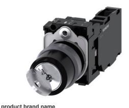
RONIS key-operated switch, 22 mm, round, plastic with metal front ring, lock number SB30, with 2 keys, 2 switch positions O-I, latching, actuating angle 90°, 10:30h/13:30h, key removal O+I, with holder, 1 NO+1 NC, screw terminal
