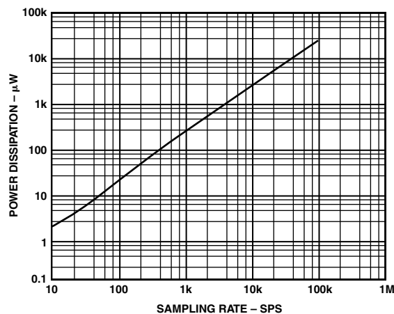
Figure 10. Power Dissipation vs. Sample Rate
