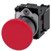
Mushroom pushbutton, 22 mm, round, plastic with metal front ring, red, 40mm, latching, pull-to-unlatch mechanism, with holder, 1 NC, screw terminal, with laser labeling, lower case
