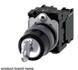
RONIS key-operated switch, 22 mm, round, plastic with metal front ring, lock number SB30, with 2 keys, 3 switch positions I-O-II, latching, actuating angle 2x45°, 10:30h/12h/13:30h, Key removal I+O+II, with holder, 1 NO, 1 NO, screw terminal, Z=20-unit packaging
