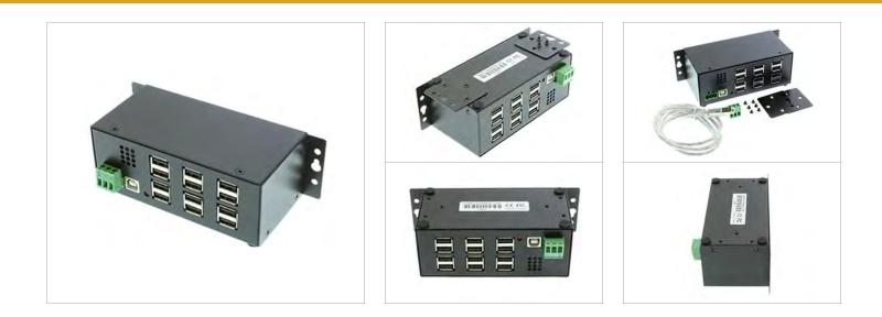
12-Port USB 2.0 powered hi-speed hub enabling you to connect 12 additional USB peripherals to your system. Industrial-grade metal chassis supporting rugged use, is backward compatible with USB 1.0/1.1. The USBG-12U2ML operates seamlessly with both Microsoft Windows and Apple Macintosh Operating Systems. As a standard USB hub, the USBG-12U2ML buffers USB data from any attached peripheral in compliance with USB specifications.
