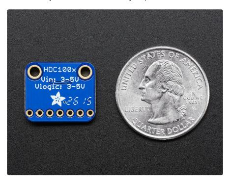
This I2C digital humidity sensor is a fairly accurate and intelligent alternative to the much simpler <u>Humidity and Temperature Sensor - SHT15 Breakout</u> (http://adafru.it/1638) It has a typical accuracy of ±4% with an operating range that's optimized from
