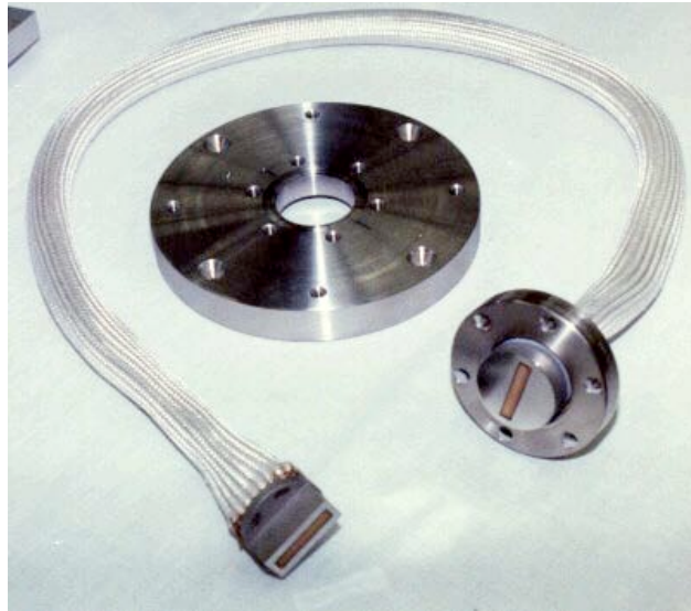
Photo 5. Optical fiber bundle enclosed in a flexible stainless steel sheath transfers light from one area to another.
