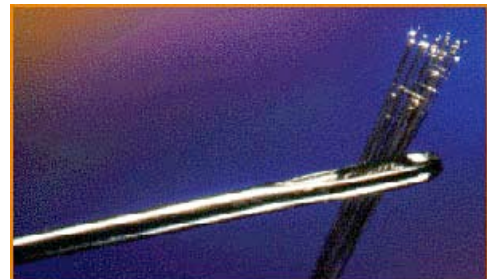
Photo 18. Glass optical fibers are very small in diameter as can be seen by the multiple fibers through this needle's eye.
