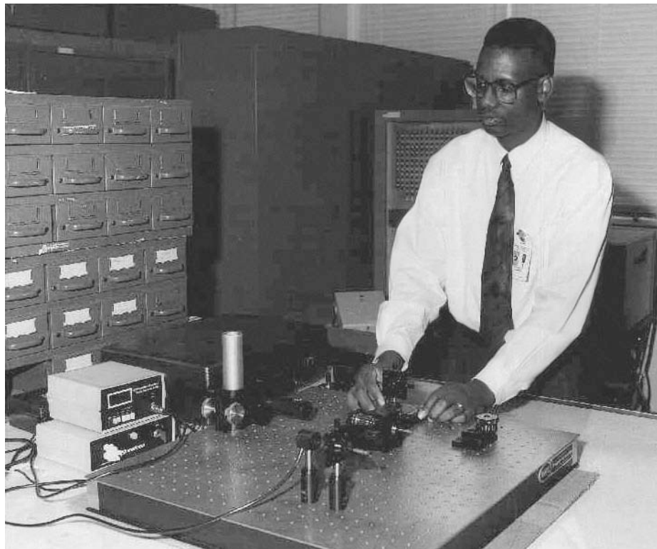
Photo 15. Researcher sets up equipment to test or characterize a fiber optic transmitter.
