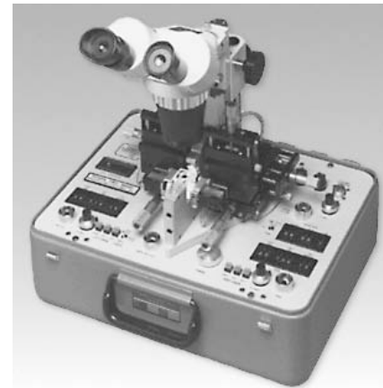
Photo 20. Fusion splice for glass optical fiber.
