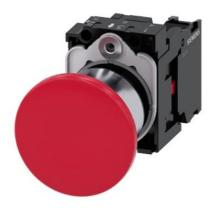
Mushroom pushbutton, 22 mm, round, metal, shiny, red, 40mm, latching, pull-to-unlatch mechanism, with holder, 1 NC, screw terminal, with laser labeling, symbol number according to, ISO 7000 or IEC 60417
