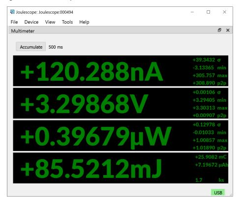
You can return to this view at any time using **View** → **Multimeter**.
