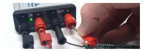
Operate your device under test. The Joulescope host software starts in the **Multimeter** view by default. Use the **Multimeter** view to measure the current, voltage, power, charge, and energy consumption.
