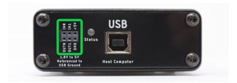
These signals enable time-synchronization with the device under test and other external equipment. The user interface can display GPIs time-synchronized with current, voltage, and power in the oscilloscope view.
