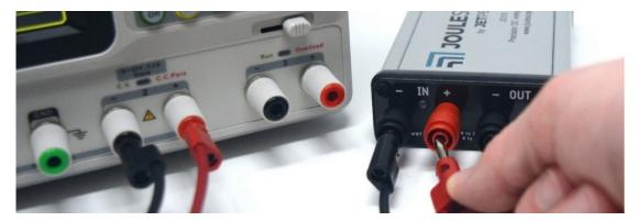
Connect the Joulescope "OUT" port to the power input for your device under test.
