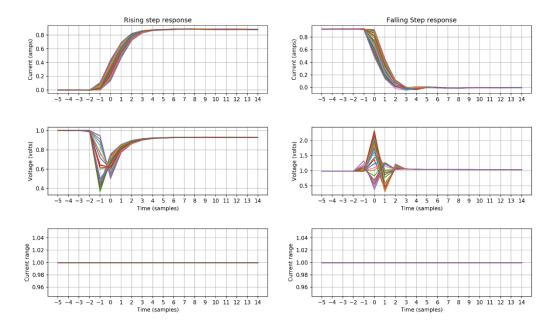
Figure 2: Step response with fixed 2A range
