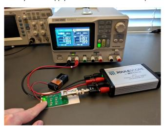
Figure 1: The step response test setup
