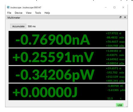
Connect the Joulescope **IN** port to your power source. If using a configurable power supply, set the voltage and current suitable for your device under test. The maximum voltage between **IN+** and **IN-** should never exceed ±15V. **IN** and **OUT** are electrically isolated from USB, but the voltage between any port and USB ground should never exceed ±48V.
