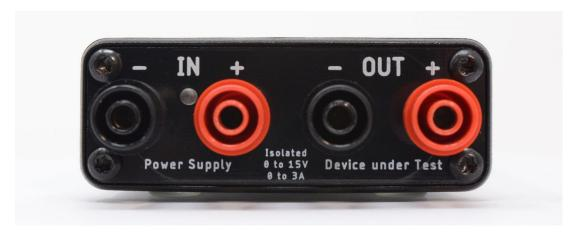
The LED indicates when your Joulescope is ready to collect measurements.
