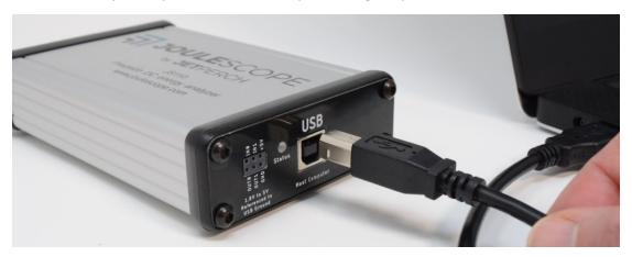
The host software will automatically detect the connected Joulescope and start displaying data.
