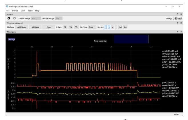
The first view allows you to control the connected Joulescope. Press to pause or resume capturing live data. Press to start and stop recording data to a file. This feature is only available when the device is capturing live data.
