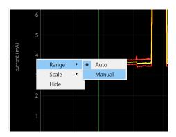
When manual ranging is activated, hover over the y-axis and use the scroll wheel to zoom in and out. Left-click and drag up and down to pan the y-axis.
