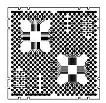
Supports 36 pins with a .5mm pitch and 32 pins with a .65mm pitch for QFN devices
