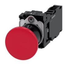
Mushroom pushbutton, 22 mm, round, plastic, red, 40mm, latching, pull-to-unlatch mechanism, with holder, 1 NO+1 NC, screw terminal, with laser labeling, upper case
