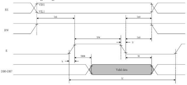
Write cycle (Ta=25°C, VDD=5.0V)
