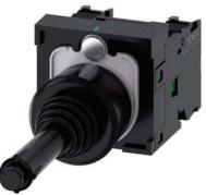
Coordinate switch, 22 mm, round, plastic, black, 2 switch positions, horizontal, momentary contact type, with mechanical interlocking in O position, with holder, 1 NO, 1 NO, screw terminal, with laser labeling, lower case
