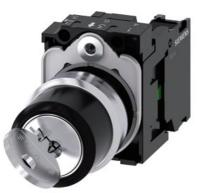
RONIS key-operated switch, 22 mm, round, metal, shiny, lock number SB30, with 2 keys, 2 switch positions O-I, latching, actuating angle 90°, 10:30h/13:30h, key removal O+I, with holder, 1 NO, screw terminal, possible special locks: SB31, 421, 455 inscription or symbol Customer-specific selection with SIRIUS ACT Configurator (CIN)
