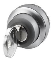
key-operated switch for extension units, 22mm, round, plastic, latching, 3 switch positions 1-0-2, 2 NO contacts, with 2 keys (incl. printed-circuit board, contact module)
