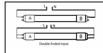
Input voltage: 120-277Vac 50/60Hz
