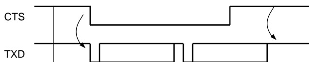
Figure 34-29. Transmitter Behavior when Operating with Hardware Handshaking
