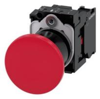
Mushroom pushbutton, 22 mm, round, plastic, red, 40mm, latching, pull-to-unlatch mechanism, with holder, 1 NC, screw terminal, with laser labeling, upper case
