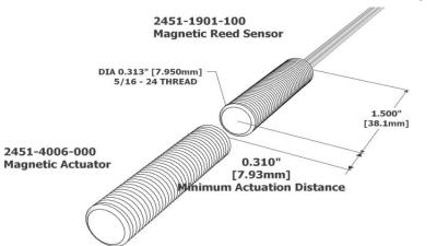
All measurements are in Inches [millimeters]
