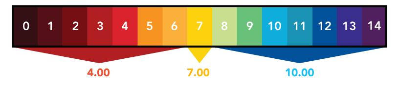
There is no correct order when calibrating to **4.00** and/or **10.00**. Recalibrating these two points will not have any effect on the other stored calibration points. Calibrating the IXIAN<sup>™</sup> pH Transmitter to **4.00** and/or **10.00** can be done at any time.
