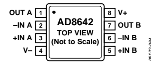
Figure 4. 8-Lead MSOP (RM-8)
