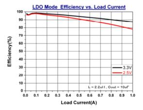
Figure 6. Efficiency vs. Load Current
