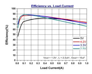
Figure 4. Efficiency vs. Output Current
