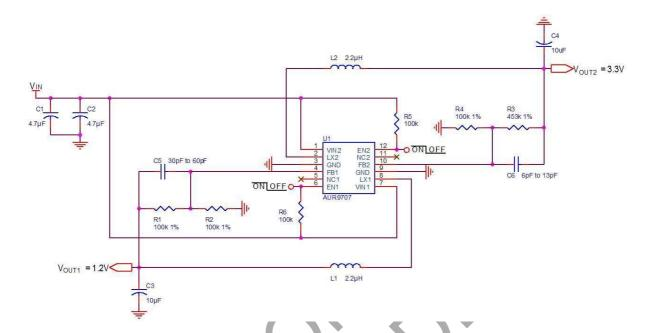
Figure 20. The Evaluation Board Schematic
