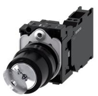
RONIS key-operated switch, 22 mm, round, plastic, lock number SB30, with 2 keys, 2 switch positions O-I, latching, 10:30h/13:30h, key removal O+I, with holder, 1 NO+1 NC, spring-type terminal, possible special locks: SB31, 421, 455, with laser labeling, upper case and lower case, always upper case at beginning of line
