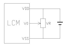
$V_{\text{DD-}}V_0$ : LCD Driving voltage
