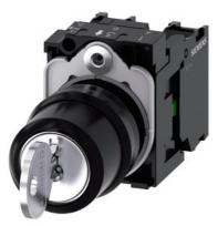
RONIS key-operated switch, 22 mm, round, plastic, lock number SB30, with 2 keys, 3 switch positions I-O-II, latching, 10:30h/12h/13:30h, Key removal I+O+II, with holder, 1 NO, 1 NO, screw terminal, possible special locks: SB31, 421, 455, with laser labeling, upper case and lower case, always upper case at beginning of line
