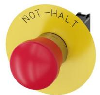
EMERGENCY STOP mushroom pushbutton, 22 mm, round, metal, shiny, red, 40 mm, positive latching, according to DIN EN ISO 13850, pull to unlatch, with yellow backing plate, inscription: NOT-HALT, with holder, 1 NC, screw terminal, Z=20-unit packaging
